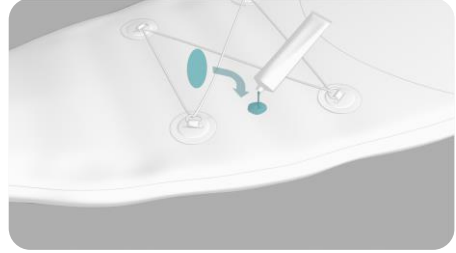
Apply one layer of glue on the patch and on the damaged area
